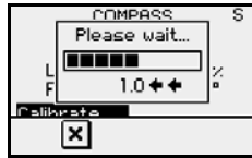
Turn rate too high, turning cw
