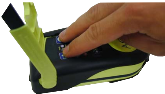
Figure 4 Activation Press both test buttons simultaneously for more than ½ second and no longer than 5 seconds
