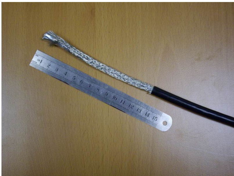
Figure 26 - Cable Jacket Removal
