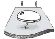
Access Under Mounting Location
