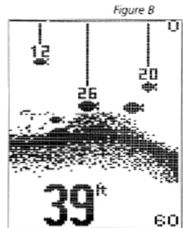
Wave action also affects the bottom depiction. Remember that the information drawn is a distance measurement, so if the boat is moving up and down over flat bottom, the bottom depiction often appears in regular variations which match wave timing.
