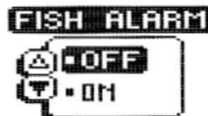
Once the Fish Alarm is enabled, the 100SX emits an audible beep when the selected size fish symbol appears on-screen. The sound is slightly different for each of the three fish symbol sizes, so with practice, it is possible to distinguish the size of the detected fish without looking at the unit.
