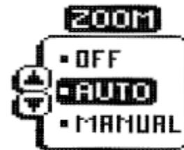
Pressing the DOWN ARROW again to highlight "Manual" activates Manual Zoom. The menu further expands to show the current Zoom range, and allows user adjustment of this range.
