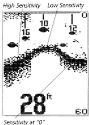
The user has the option of biasing this Sensitivity adjustment either higher or lower based on personal preference. You can select one of 11 sensitivity bias settings from -5 to +5. A bias setting of 0 (Factory Setting) has no effect on the automatic sensitivity control. Increasing the bias (+1 through +5) causes the unit to display the information from progressively smaller sonar returns. By decreasing the sensitivity bias (-1 through -5), the unit effectively filters small sonar returns.
