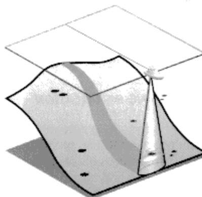
Sonar is very fast. A sound wave can travel from the surface to a depth of 240' (70m) and back again in less than 1/4 of a second. It is unlikely that your boat can "outrun" this sonar signal.
