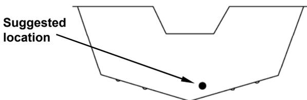
**To install the EP-80R TH, use a hole saw to cut a 1-1/16" (27 mm) hole in the transom. The hole should be below the waterline.**
