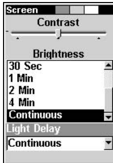
Light Delay menu. Setting shown is "Continuous," which is ideal for night travel in a vehicle on external power.
