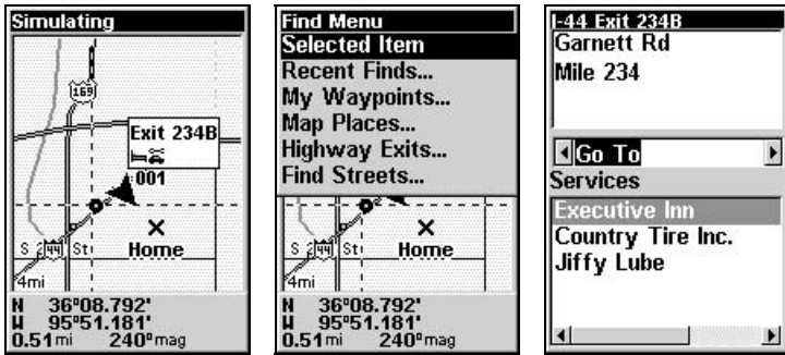
A highway exit selected by the cursor, left, The Find Menu, center, Waypoint Information screen, right.
