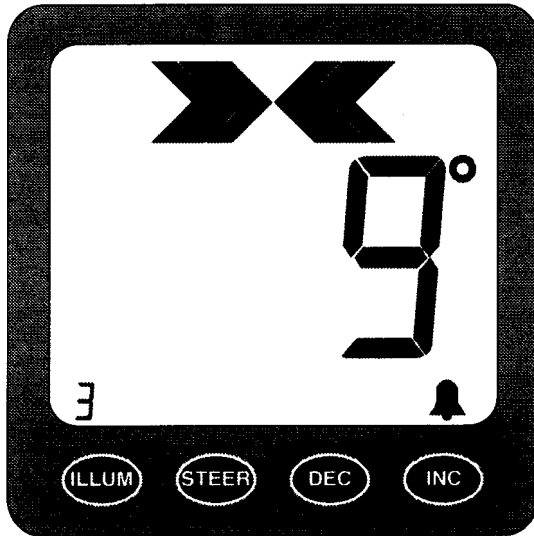
FIGURE 6 - Alarm Boundaries set at +/- 9°
