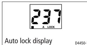
Whenever the autopilot is engaged, the heading set by the autopilot is displayed on the digital display and the analogue pointer displays the autopilot's course error.
