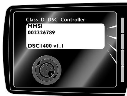
Fig 4.5 - Displaying MMSI & software version
