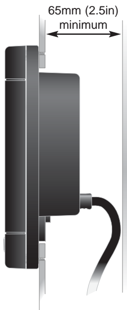
Fig 4.2 - Clearance Required Behind Bulkhead
