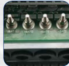
The DC connection on threaded rods is particularly robust and practical due to the available space.
